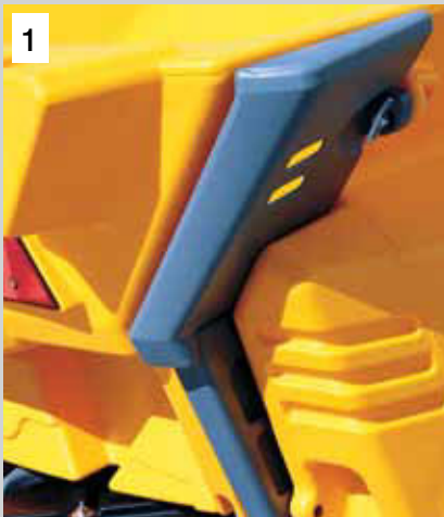
1 Release the catch with a gloved hand.
