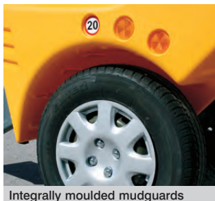
Integrally moulded mudguards
