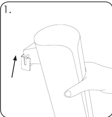
1. To transport the Cup Tube, lift the tube off the Cup Stacker Bracket.
