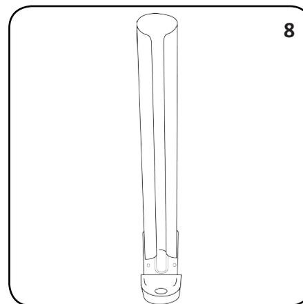
Place ITEM 5 onto the Cup Stacker Bracket and place ITEM 6 onto the Drip Tray Bracket.
