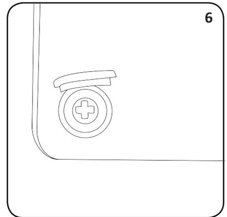
Place the A4 Foamex Sign against the 4 fixings holes and thread one of the Screw fixings into the wall plug. Fit all 4 fixings, using the Screwdriver to tighten.
