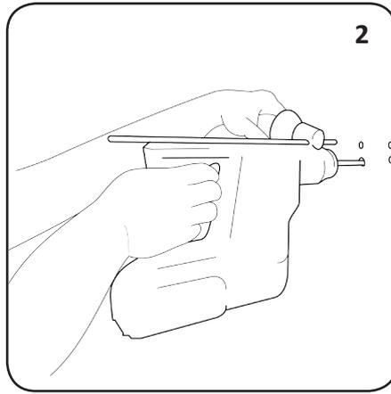
Drill the 4 marked points with the Hand Drill. Repeat steps 1&2 for the Drip Tray Bracket holes. There should be 656mm between the base of ITEM 1 and the top of ITEM 4.
