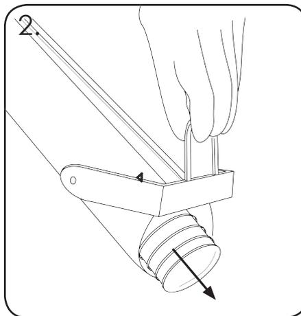
2. Using the Stainless Steel ring, open the Quick Release Mechanism to remove cups.
