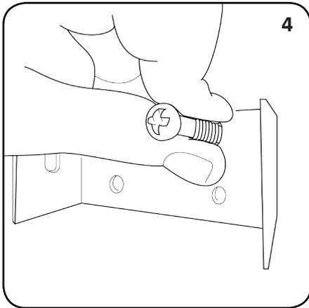
Place the Cup Stacker Bracket against the top 4 fixings holes and thread through ITEM 3.
