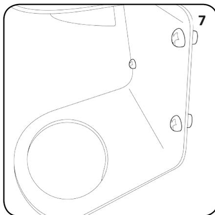
Repeat step 6 for all 4 fixing points securing the Drip Tray Bracket to the wall.
