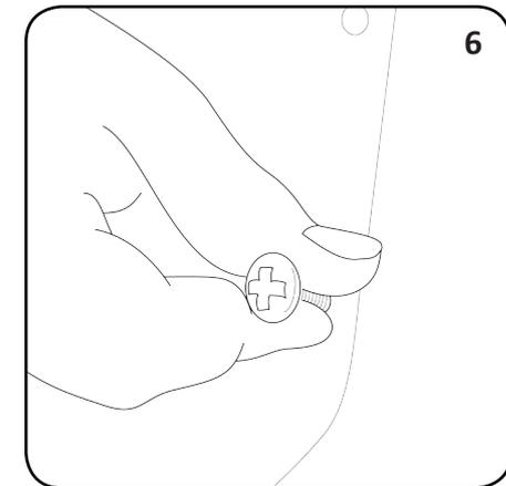
Place ITEM 4 against the wall aligning the 4 holes with the 4 wall plugs, Thread through one of the SCREWS and tighten with the Screwdriver.
