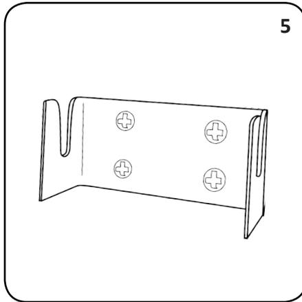
Tighten the Screw with the Screwdriver and repeat for all 4 fixings points securing the Cup Stacker Bracket to the wall.
