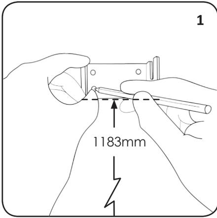
Using the 'Fixing Point Guide' as a reference, measure 1183mm from the ground level and mark with the pencil. Align the base of ITEM 1 with the line against the wall and mark the hole positions.
