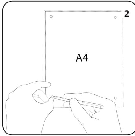
Place ITEM 1 against the wall 60mm above the top of ITEM 5. Mark 4 fixing points on the wall through the 4 holes in the A4 Foamex Sign, ensure the sign is horizontal and centrally straight.
