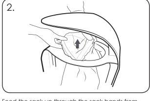
Feed the sack up through the sack bands from beneath. Wrap the top of the sack over both bands.
