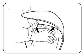
Lift the two sack bands upwards.
