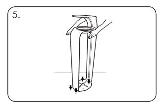
Reposition the bin over the drilled holes.
