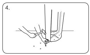
Hammer in the anchor sleeves [ITEM 4] into the drilled holes until the top of the sleeve is level with the ground.
