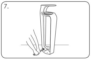
Tighten the bolts into the ground using a 17mm spanner or socket set.
