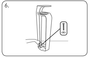
Insert the bolts through the ground fixing holes in the bin into the anchor sleeves in the ground. Tighten by hand to start with.
