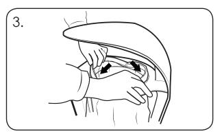
Push the sack bands down to trap the sack between the bands and the sack ring, clamping it in an open position ready for use.
