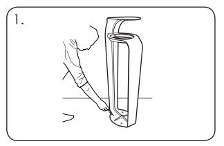
Position the bin [ITEM 1]. Using a pen mark the positions of the four ground fixing holes in the base onto the ground below.
