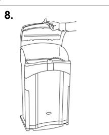
Pivot the lid forward so it locates over the door to secure the unit.
