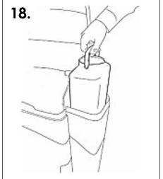
Using the handle on the reservoir, remove from the side pod to empty.
