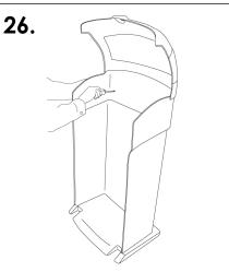
From the inside of the unit attach the sign carrier to your Nexus 100 with the use of the five screws provided.
