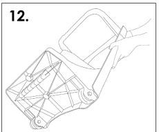
Two casters are located at the front of the door which allow it to be tilted and wheeled from the body providing excellent access to the contents and for cleaning.
