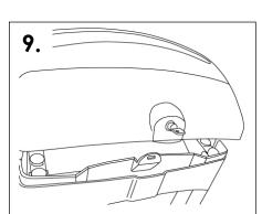
The Confidential Paper model comes complete with a push lock which is located at the front of the unit. With the lid shut, push the lock centre to lock the unit (the lock is available as an optional extra on all models).
