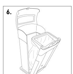
Fold the sack around the sack retention band so the sack is held securely then close the door followed by the lid.
