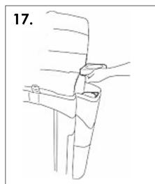
The funnel is then removed from the side pod for ease of access and cleaning.
