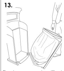
The door can now be utilised to transport heavy waste (i.e. paper a short distance to a collection area.
