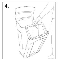
Once the door is tilted forward the sack retention band is exposed.
