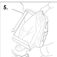
Install the correct size sack (406 x 727 x 1093mm-available from Glasdon) by firstly hooking onto the retention lugs at the front of the door.
