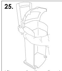
After opening the unit and removing the door. Position the sign carrier at the rear of the unit and align the five fixing holes.
