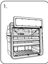
Locate the fixings on each end of the metal support bar that attach to the inside of the body.
