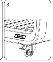
To release the brake push down on the smaller lever.
